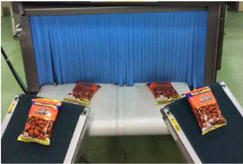
Dual lane x-ray machine can inspect contaminants in products feeding from 2 packaging lines
